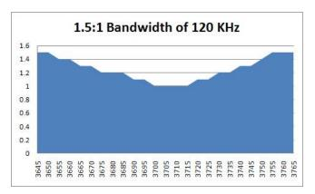
• 1.5:1 bandwidth of 120 KHz—from 3.645 to 3.765 MHz
