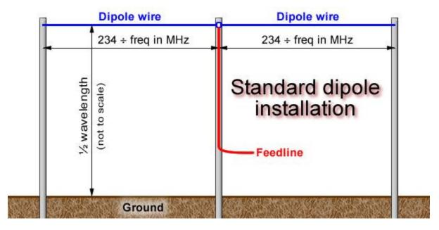
On the other hand, an NVIS dipole works best when mounted 0.05 wavelengths above the ground: about 13 feet for 80m or 7 feet for 40m. To make an NVIS dipole work even better, you can mount a reflector wire (that is 5% longer than than the total dipole length) at 0.02 wavelengths above the ground: about 5 feet for 80m or 3 feet for 40m. This basically turns the antenna into an upward pointing yagi.
