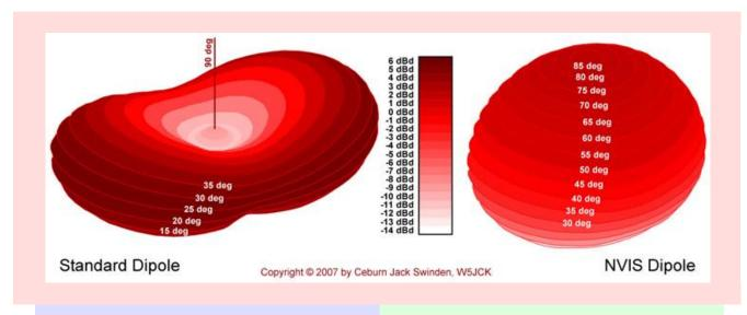
The following is a brief comparison of a standard 1/2 wavelength dipole and a 1/2 wavelength NVIS dipole with a reflector wire (5% longer than the total length of the dipole) mounted below it.
