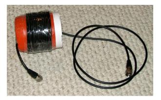
I used a short 10 foot (3 meter) piece of RG-58 coax to make my RF choke balun. I connected the short end of the RF choke balun to my antenna, and the other end was connected to a 50 foot (15 meter) RG-8 coax cable that runs to the tuner in my shack. This method allows me to use the RF choke balun with any coax cable, which is handy for portable use.
