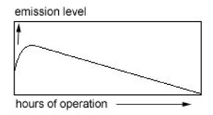
Above is a graphic representing the emission level verses hours, of a typical power tube. The graph is not to scale, the hours side is 12K hours.
