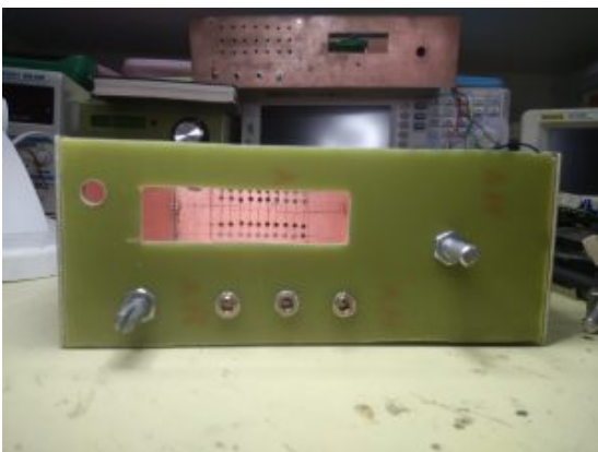
The front panel controls are installed.
