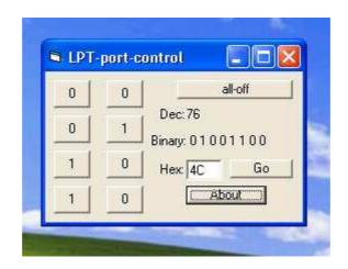
Using buttons you can turn ON and turn OFF all eight relays.
