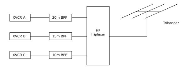
**Note:** You cannot use a high power amplifier before or after the HF Triplexer!
