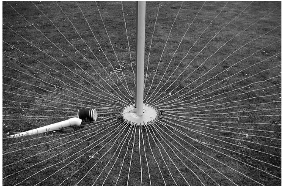
Figure 5 — Here is the test antenna base at ground level, with 64 radials.
