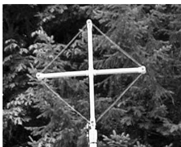
Figure 7 — This photo shows the loop receiving antenna.
