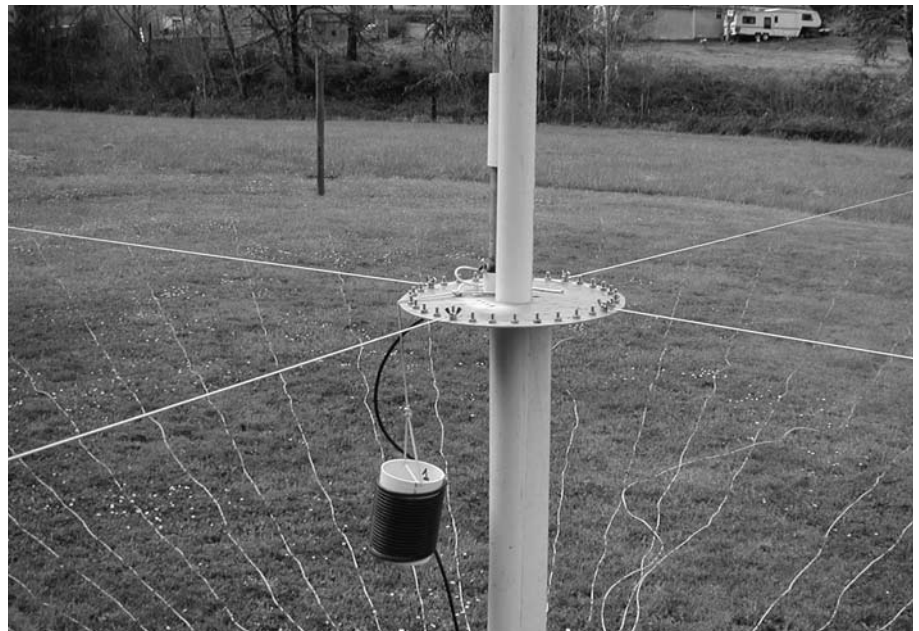
Figure 6 — The base plate is in position for elevated radials.
