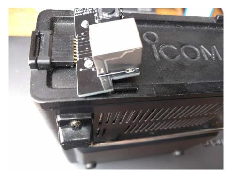
2. Push the base unit adapter and fix it with a thumb screw:
