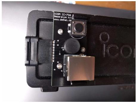
4. Check that pogo pins points exactly to the edge connector of the base unit adapter:
