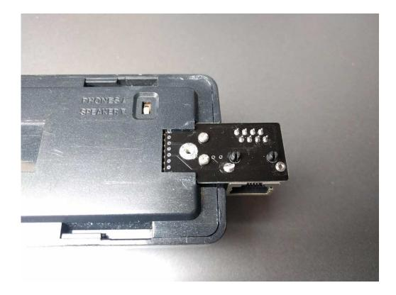
6. Insert RJ-45 cable and power the device on.
